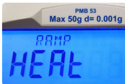
Four preset drying methods allow test routines for a wide variety of samples
