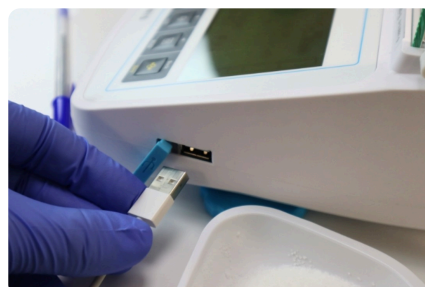
Built-in Bluetooth, ethernet, RS-232 and USB interfaces for enhanced recordkeeping
