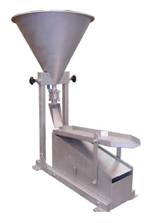
The Magna Chute is used for the determination of Magnetite or Ferro-Silicon losses in Wet Drum Separator Tailings.
